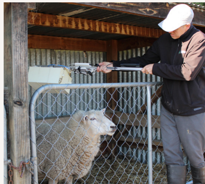
Our innovative tool uses radar to measure fat depth.
