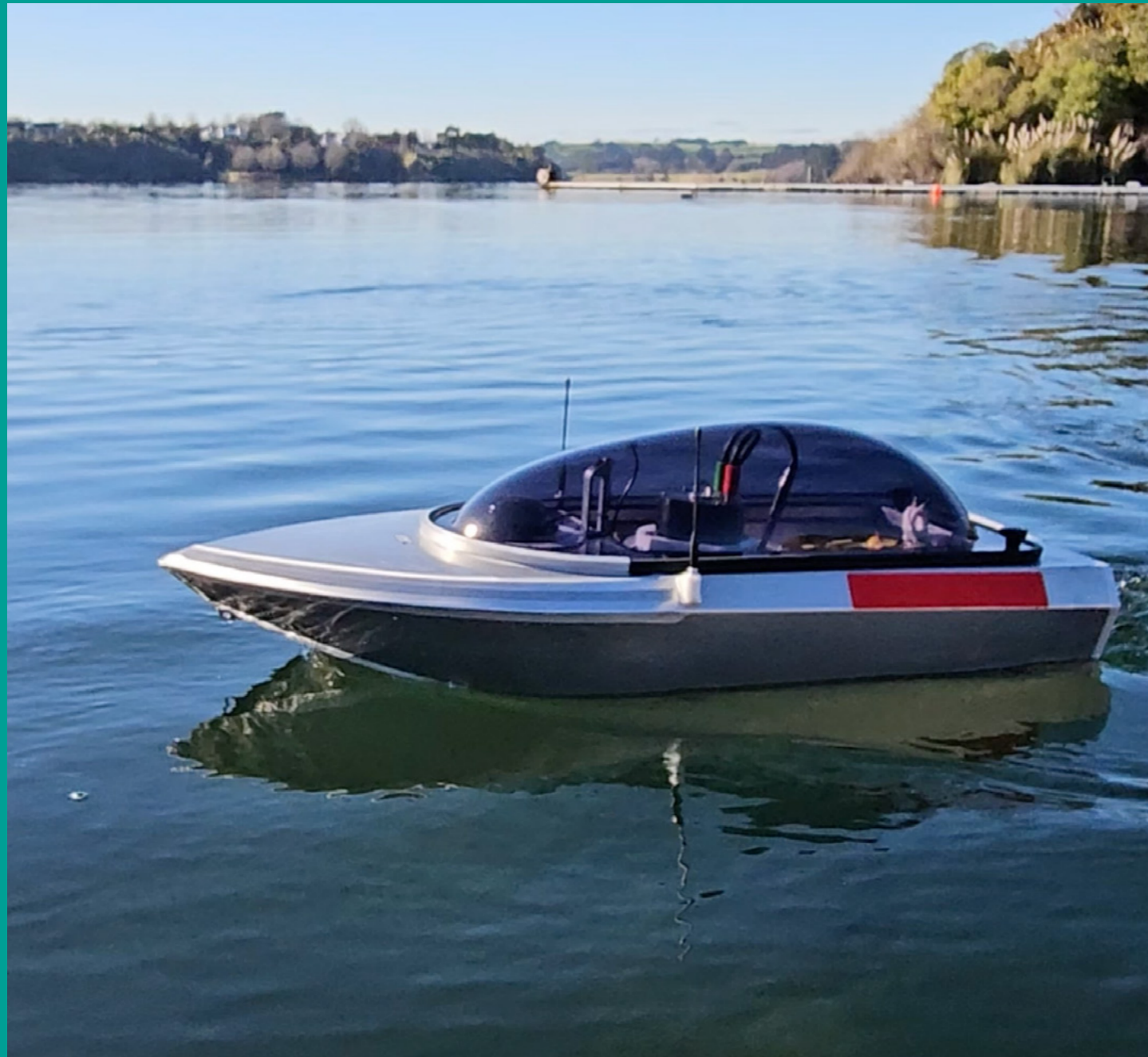
Quarter-scale jet boat designed specifically for remote monitoring of waterways.
