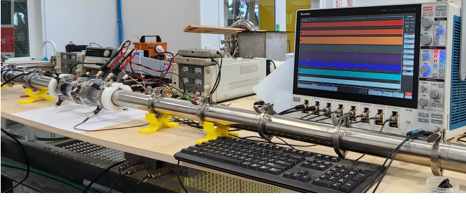
Fig. 6. Photo of the dual sensor installed in the recirculating test rig. The sight-glasses can be seen in the left foreground.
