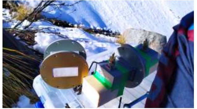
Fig. 3. Microwave waveguide measurement of snow in the field with snow sample, extracted using an open ended plastic sample holder, is inserted into the waveguide section.
