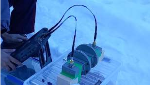
Fig. 2. Measurement setup where the two ports of the snow-filled waveguide section is connected to the vector network analyser via adaptors and coaxial cables.
