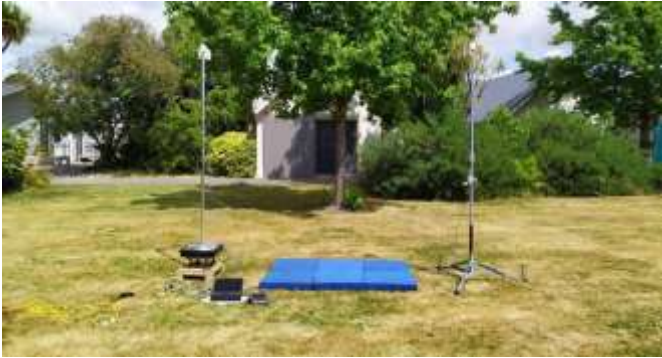
Figure 4. Photo of the open range measurement setup for antenna gain pattern measurements.
